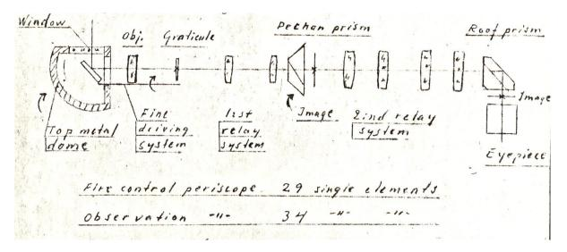
When the top unit rotates to point round the horizon, the image rotates. This is compensated by a special prism, rotating with half the speed. In this case a Pechan prism was chosen which can be located in convergent light and requires small room.
