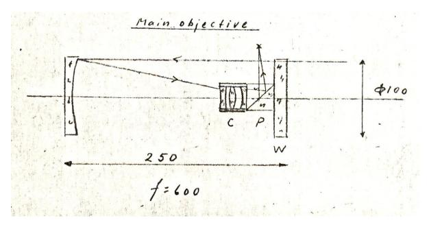
The focal length of the objective was 600 mm, but the building length only 250. The correction system C had two tasks
