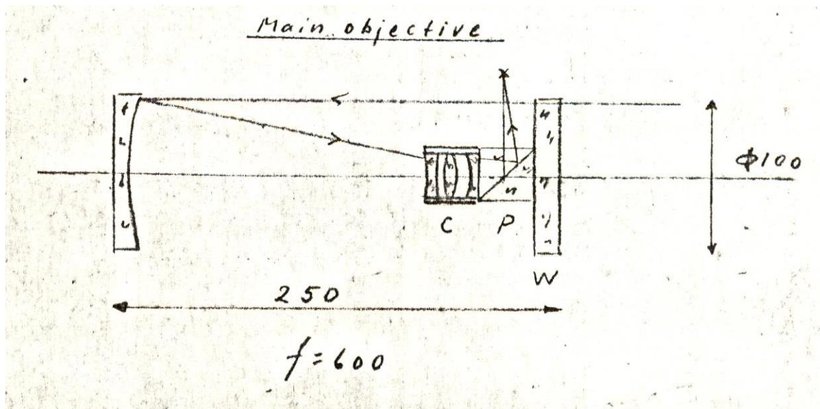
The focal length of the objective was 600 mm, but the building length only 250. The correction system C had two tasks
