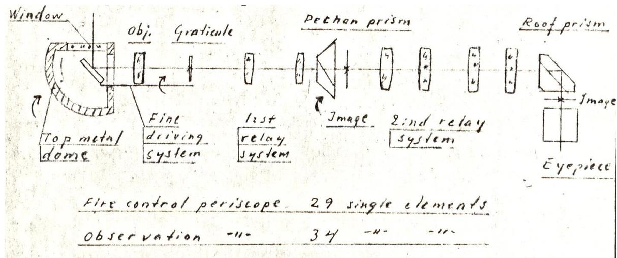
When the top unit rotates to point round the horizon, the image rotates. This is compensated by a special prism, rotating with half the speed. In this case a Pechan prism was chosen which can be located in convergent light and requires small room.
